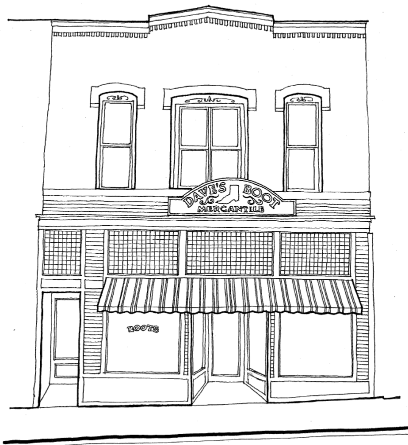
Figure 11 Awnings can be located below the transom if the display window is tall enough.
