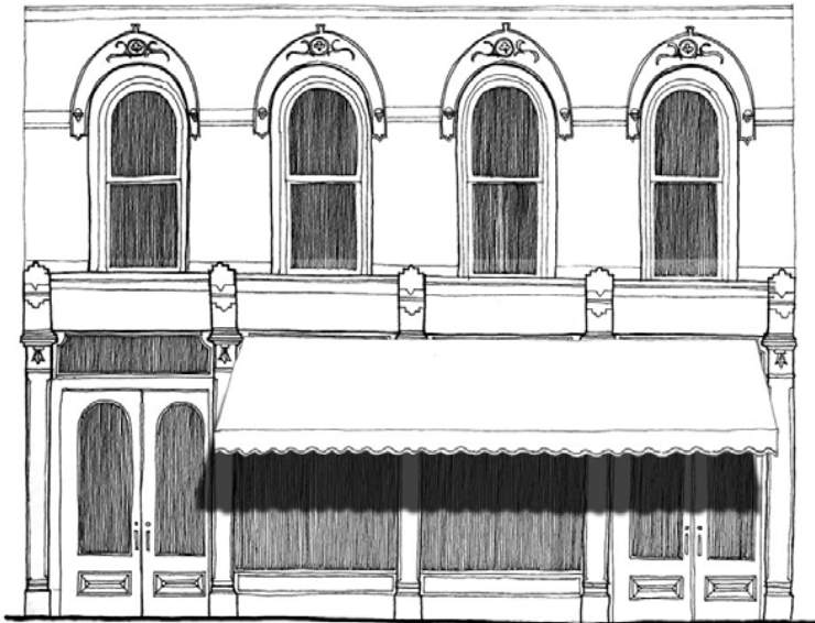
Figure 13 Building features should not be covered by awnings
